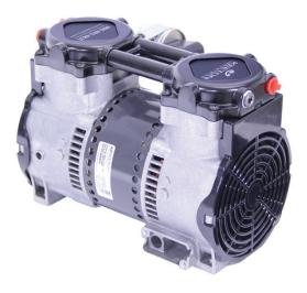
AerFlow<sup>™</sup> Rocking Piston Compressor features a powerful compressor capable of delivering 5.3 CFM and 50 PSI while maintaining low vibration, whisper quiet operation. The AerFlow<sup>™</sup> is made from a die cast aluminum, thin-walled, anodized cylinder. Its unique, corrosion resistant design and thermal overload protection ensures a long and service free operational life. The AerFlow<sup>™</sup> Rocking Piston Compressor fits all ProLake<sup>™</sup> lake bed aeration models.
